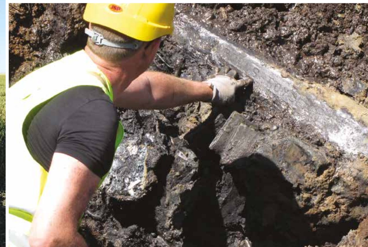
Above: Appearing out of the mud is the Defiant's Merlin engine complete with the Rolls-Royce name on the engine block. A couple of exhaust stacks can be seen below the name.
