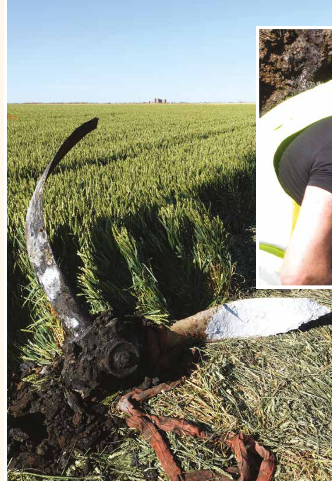
Above: Appearing out of the mud is the Defiant's Merlin engine complete with the Rolls-Royce name on the engine block. A couple of exhaust stacks can be seen below the name.
